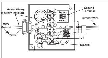
Figure 56. Electrical Wiring - Junction Box
