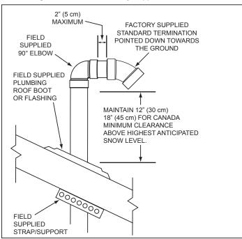
Figure 22. Vertical Termination(s) Installation
