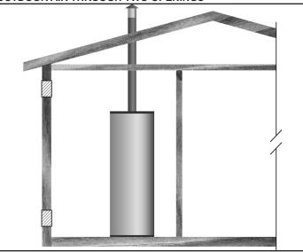
Figure 9. Outdoor Air Through Two Openings
