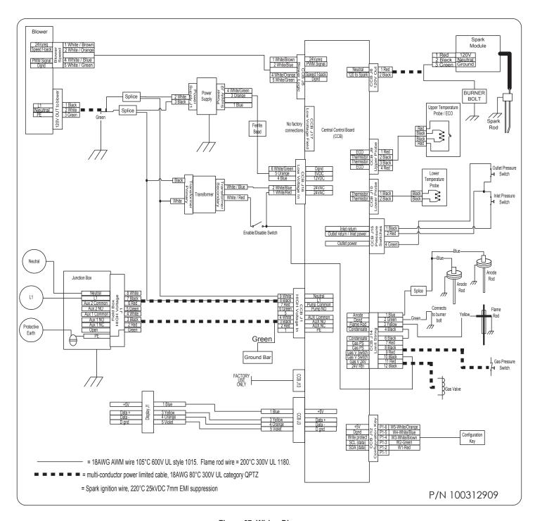
Figure 67. Wiring Diagram
