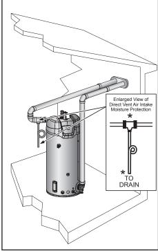
Figure 48. Direct Vent Vertical Concentric
