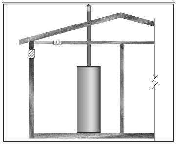
Figure 10. Outdoor Air Through One Opening
