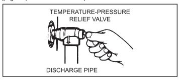
Figure 65. Testing the T&P Relief Valve
