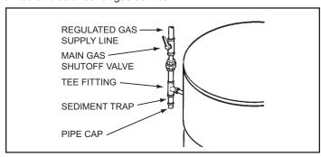
Figure 54. Supply Gas Line Installation
