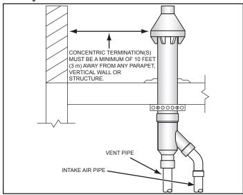
Figure 27. Concentric Termination - Flat Roof Clearance
