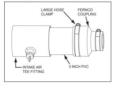
Figure 16. Intake Air Connection Pipe
