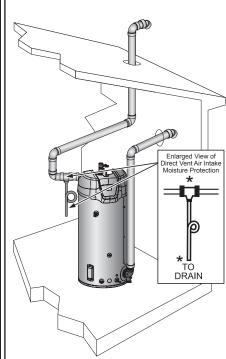
Figure 45. Direct Vent Horizontal
