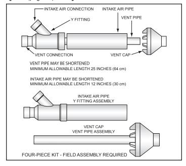
Figure 28. Concentric Termination Kit
