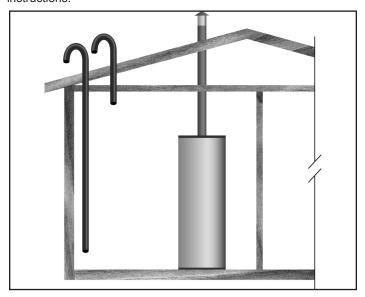
Figure 12. Two Vertical Ducts
