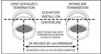
Figure 25. Side-Wall Termination - Direct Vent
