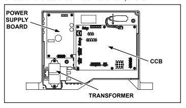
Figure 58. Control System Components
