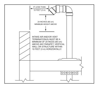
Figure 23. Vertical Termination Flat Roof Clearance - Intake Air and/or Vent (exhaust)
