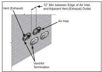
Figure 41. Multiple Low-Profile Vent Clearance
