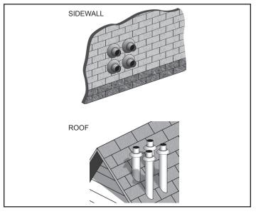
Figure 37. Four Concentric Terminations
