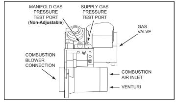
Figure 60. Gas Valve/Venturi Assembly Top View
