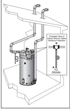
Figure 42. Power Vent Vertical
