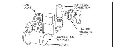
Figure 62. Gas Valve/Venturi Assembly Side View
