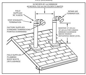
Figure 24. Vertical Termination - Direct Vent
