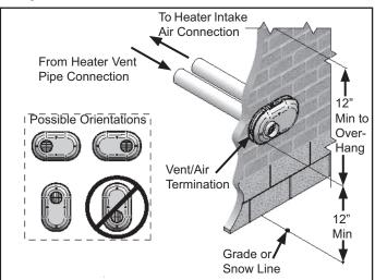
Figure 40. Low-Profile Vent Clearances
