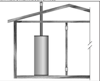
Figure 13. Two Permanent Openings
