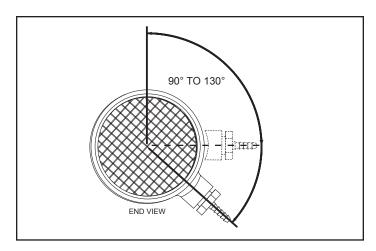
Figure 15. Orientation of Intake Air Tee Fittings
