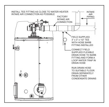
Figure 20. Intake Air Condensate Tee Installation
