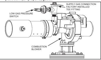
Figure 55. Supply Gas Line Connection
