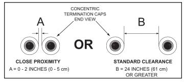
Figure 31. Two Concentric Terminations
