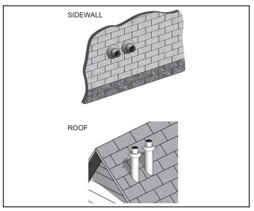
Figure 36. Two Concentric Terminations
