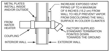
Figure 26. Side-Wall Termination Installation
