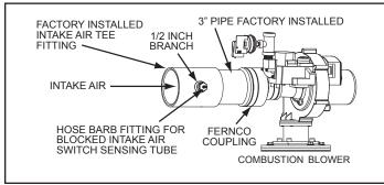
Figure 19. Intake Air Connection
