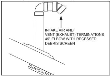
Figure 21. Standard Factory Supplied Terminations
