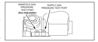
Figure 61. Gas Valve Top Detail View
