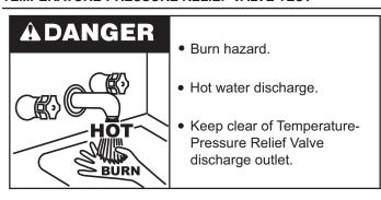
It is recommended that the Temperature-Pressure Relief Valve should be checked to ensure that it is in operating condition every 6 months.
