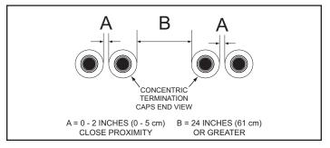
Figure 34. Four Concentric Terminations
