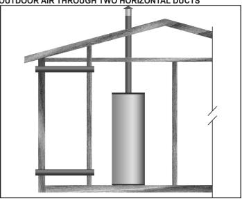
Figure 11. Two Horizontal Ducts
