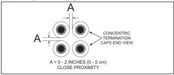
Figure 33. Four Concentric Terminations
