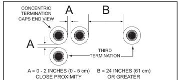
Figure 32. Three Concentric Terminations
