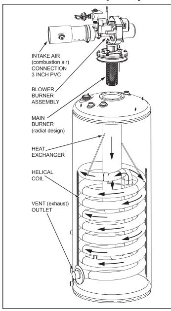
Figure 1. Water Heater Components
