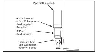
Figure 17. Vent (Exhaust) Connection
