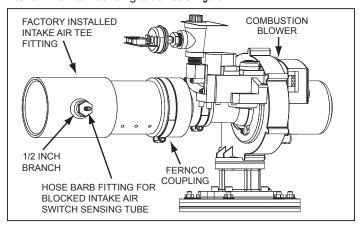
Figure 14. Combustion Blower Assembly
