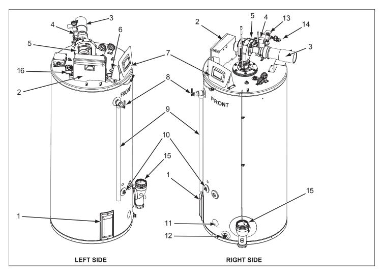
Figure 4. Left-Side and Right-Side Components
