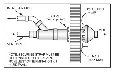
Figure 30. Concentric Termination Clearances - Side-Wall Installation
