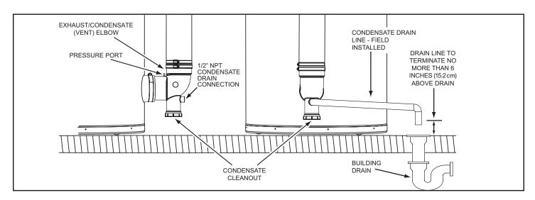
Figure 53. Condensate Drain Installation
