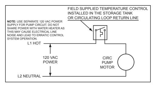
Figure 68. Circulating Pump Wiring Diagram - Storage Tank or Building Recirculation
