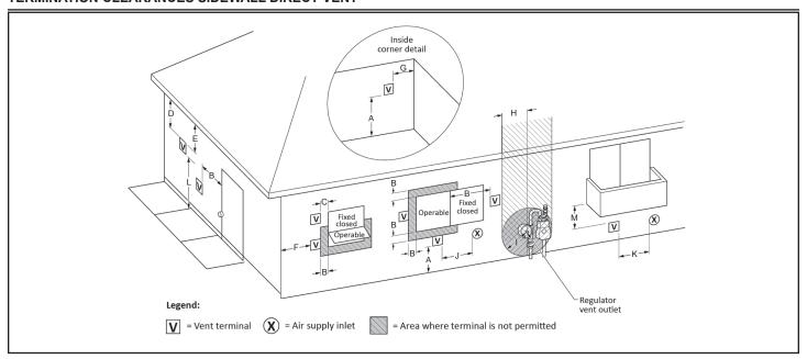
Figure 52. Sidewall Direct Vent Using Outside Air
