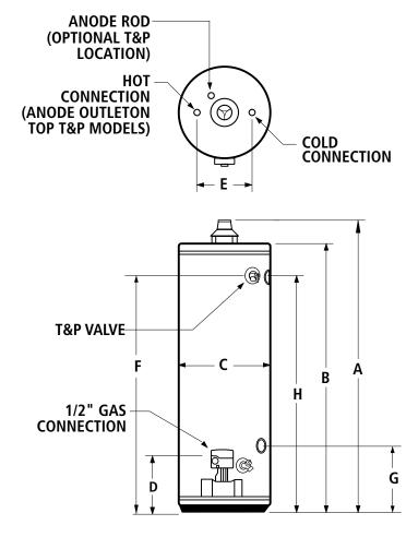
**Maximum Hydrostatic Working Pressure: 150 PSI**
