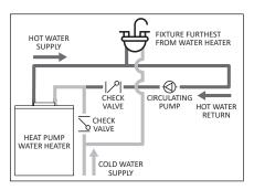
Figure 19 - Recirculation Loop Diagram
