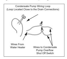
Figure 14 - Wiring Loop for connection to Condensate Pump.
