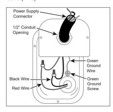
Figure 21 - Connecting the electrical wires (bottom cover to electrical junction box removed for clarity).
