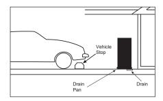
Figure 9 - In a garage, install a vehicle stop to avoid water heater damage.
