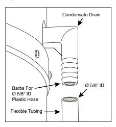
Figure 4 - Condensate drain connection
