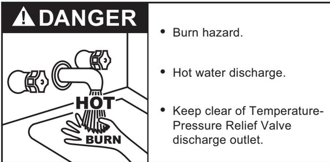
The Temperature-Pressure Relief Valve on the water heater must be manually operated at least once a year.
