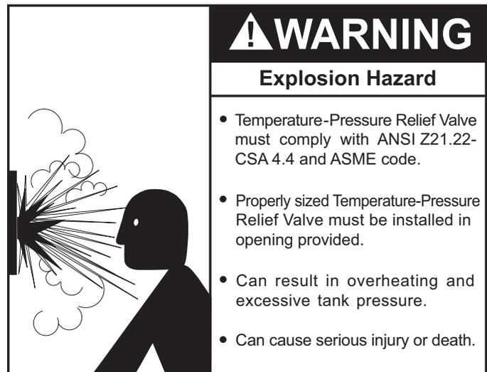
**Note:** Do not plug the Temperature-Pressure Relief Valve opening. This can cause property damage, serious injury or death.
