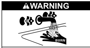
Water temperature over 125°F can cause severe burns instantly or death from scalds.
