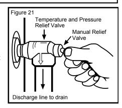
drain. Standing clear of the outlet (discharged water may be hot), slowly lift and release the lever handle on the temperature and pressure relief valve to allow the valve to operate freely and return to its closed position. If the valve fails to completely reset and continues to release water, immediately shut off the manual gas control valve and the cold water inlet valve and call a qualified person.
