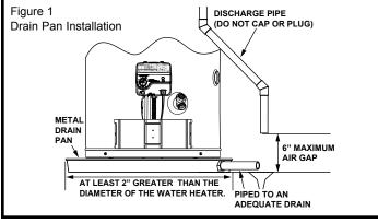
The water heater should be located in an area not subject to freezing temperatures. Water heaters located in unconditioned spaces (i.e., attics, basements, etc.) may require insulation of the water piping and drain piping to protect against freezing. The drain and controls must be easily accessible for operation and service. Maintain proper clearances as specified on the data plate.
