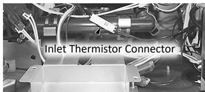
Figure 60: Inlet Thermistor Connector.
