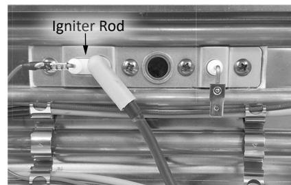
Figure 54: Igniter Rod Connections.
