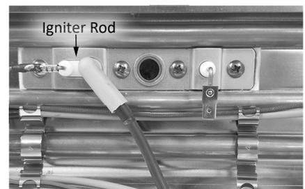
Figure 69: Igniter Rod Connections.
