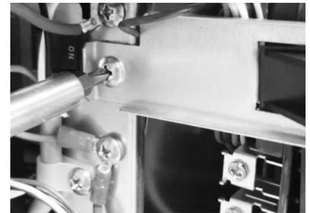
Figure 55: Computer Board Bracket.
