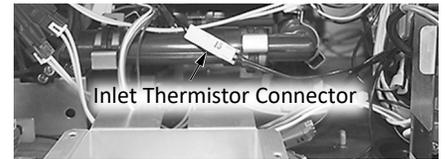
Figure 44: Inlet Thermistor Connector.
