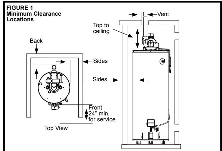
NOTE: Minimum clearances from combustible materials are stated on the data plate adjacent to the gas control valve/thermostat of the water heater.
