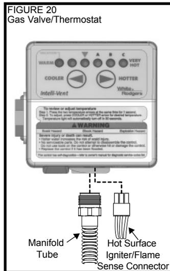
5. Grasp the manifold tube and push down slightly to free the manifold from the gas control valve/ thermostat.
