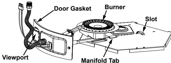
4. Inspect the door gasket and make sure there is no fiberglass insulation between the door gasket and the combustion chamber.
