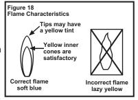
are satisfactory. The tips of the flame may have a slight yellow tint. The flame should not be all yellow or have a sharp blue-orange color. Contaminated air may cause an orange colored flame. Contact a qualified service technician if the flame is not satisfactory.
