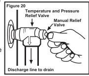
allow the valve to operate freely and return to its closed position. If the valve fails to completely reset and continues to release water, immediately shut off the manual gas valve and the cold water inlet valve and call a qualified service technician.
