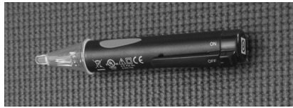
Figure 30 - Non-Contact Circuit Tester
