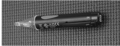
Figure 23 - Use a non-contact circuit tester to check for electrical power.
