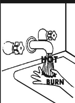
**⚠ DANGER** Water temperature over 125°F (52°C) can cause severe burns instantly resulting in severe injury or death.
