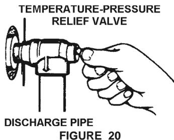
If after manually operating the valve, it fails to completely reset and continues to release water, immediately close the cold water inlet to the water heater, follow the draining instructions, and replace the temperature-pressure relief valve with a new one.
