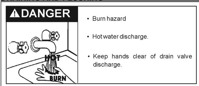
It is recommended that the tank be drained and flushed every 6 months to remove sediment which may build up during operation. The water heater should be drained if being shut down during freezing temperatures. To drain the tank, perform the following steps:
