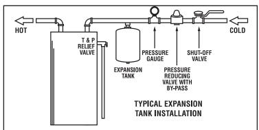
Expansion tanks are pre-charged with a 40 PSI air charge. If the inlet water pressure is higher than 40 PSI, the expansion tank's air pressure must be adjusted to match that pressure but must not be higher than 80 PSI.
