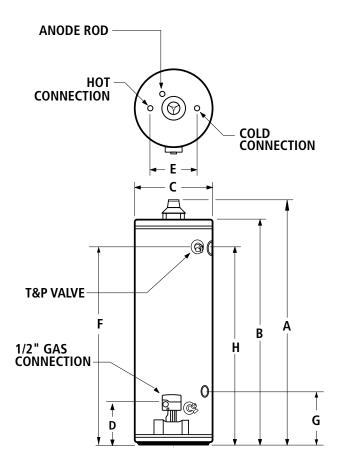
Maximum Hydrostatic Working Pressure: 150 PSI
