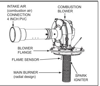
Figure 2. Blower/Burner Components
