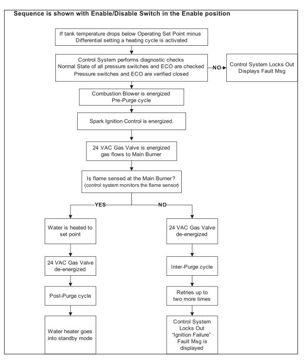
Figure 58. Sequence of Operation
