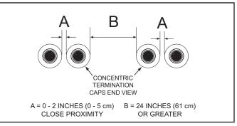
Figure 31. Four Concentric Terminations in a Line
