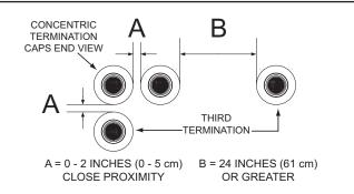
Figure 29. Three Concentric Terminations
