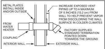
Figure 23. Sidewall Termination Installation
