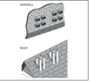
Figure 35. Eight Concentric Terminations - Sidewall and Roof
