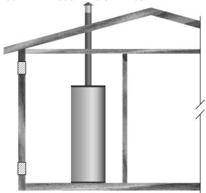
Figure 10. Outdoor Air Through Two Openings
