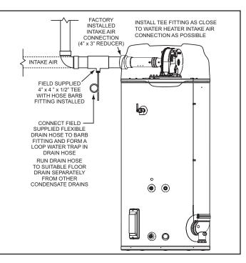
Figure 16. Intake Air Condensate Tee Installation
