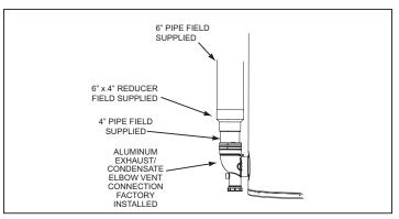
Figure 15. Vent Exhaust Connection
