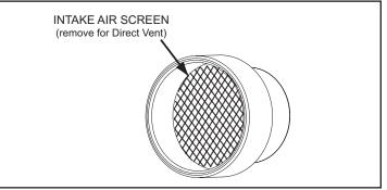
Figure 17. Intake Air Screen
