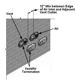
Figure 38. Multiple Low Profile Vent Clearances
