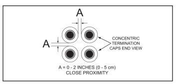
Figure 30. Four Concentric Terminations - Close Proximity
