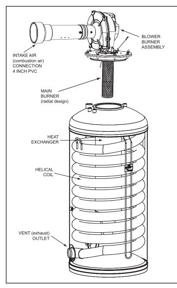
Figure 1. Water Heater Components
