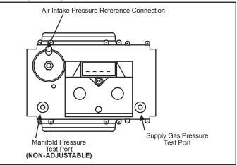
Figure 57. Gas Valve Assembly
