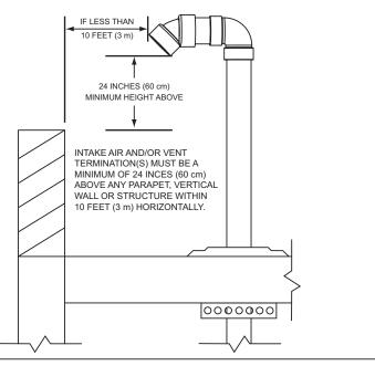
Figure 20. Vertical Termination(s) Flat Roof Clearance
