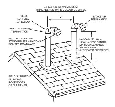
Figure 21. Vertical Termination - Direct Vent
