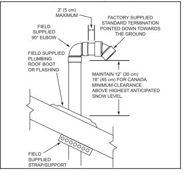
Figure 19. Vertical Termination(s) Installation
