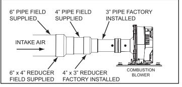
Figure 18. Intake Air Connection
