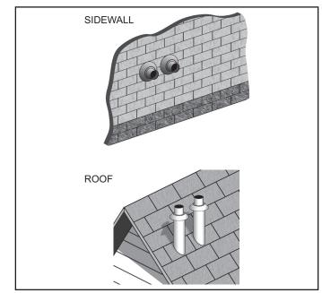
Figure 33. Two Concentric Terminations - Sidewall and Roof
