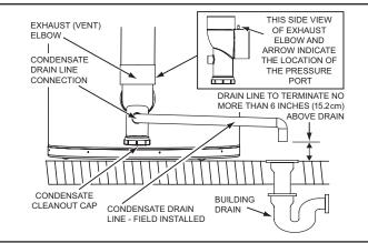
Figure 9. Exhaust/Condensate Elbow
