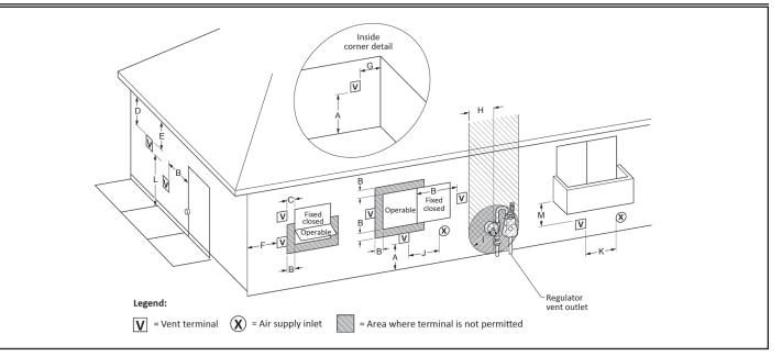
Figure 48. Sidewall Power Vent Using Outside Air
