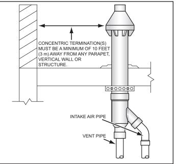
Figure 24. Six-inch Concentric Termination - Flat Roof Clearance
