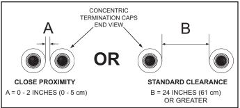
Figure 28. Two Concentric Terminations
