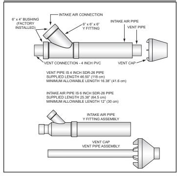
Figure 25. Six-Inch Concentric Termination Kit
