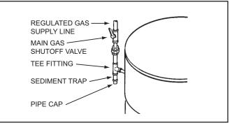
Figure 51. Supply Gas Line Installation
