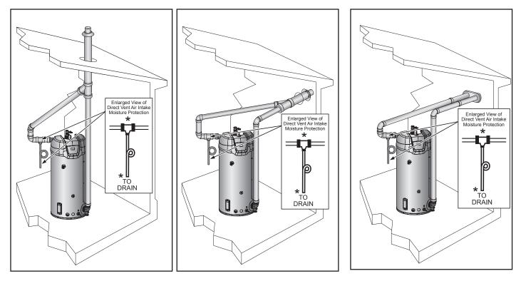
Figure 45. Direct Vent Vertical Concentric
