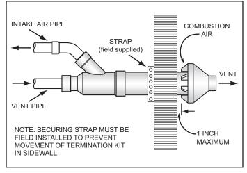
Figure 27. Six-Inch Concentric Termination - Sidewall Installation
