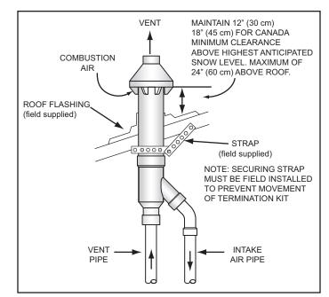
Figure 26. Six-Inch Concentric Termination - Vertical Installation
