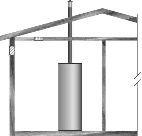
Figure 11. Outdoor Air Through One Opening
