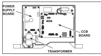
Figure 55. Control System Components
