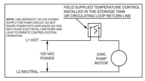
Figure 63. Recirculating Loop with Storage Tank or Building Recirculation
