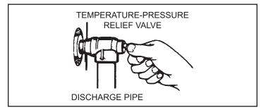
Figure 60. Testing the T&P Relief Valve
