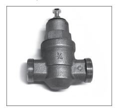
Figure 15 - A Pressure Reducing Valve is required if your home's water pressure is above 80 psi.
