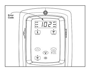
Figure 25 - Control Assembly Diagnostic Coding
