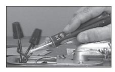
Figure 40 - Non-Contact Circuit Tester
