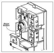
Figure 26 - Emergency Cut Off (ECO) Button
