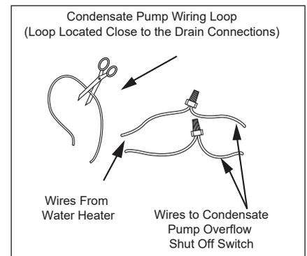
Figure 14 - Wiring Loop for connection to Condensate Pump.
