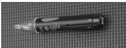
Figure 39 - Non-Contact Circuit Tester.
