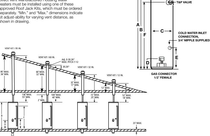
\*Inlet air pipe included 3"diameter for 30 gallon and 40 gallon. 4" diameter for 50 gallon
