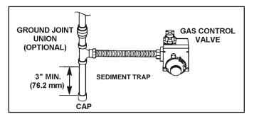
FIGURE 13. GAS PIPING WITH FLEXIBLE CONNECTOR.
