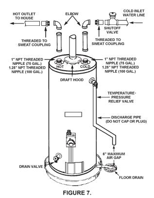
NOTE: To protect against untimely corrosion of hot and cold water fittings, it is strongly recommended that di-electric unions or couplings be installed on this water heater when connected to copper pipe.
