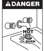
Water temperature over 125°F (52°C) can cause severe burns instantly resulting in severe injury or death.
