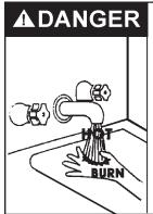
Water temperature over 125°F (52°C) can cause severe burns instantly resulting in severe injury or death.
