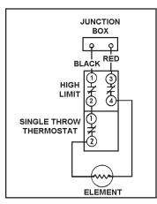
Figure 1. Two-Wire C-2 Circuit for Single-Element Heaters
