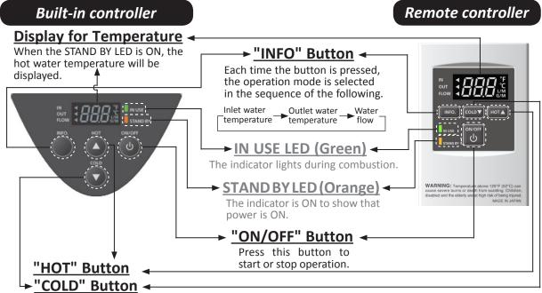
Press the "HOT" button or the "COLD" button to set the hot water temperature.
