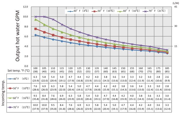
When the set temperature is 130 °F (55 °C) or higher, maximum flow rate is limited to 8.0 GPM (30.3 I/m).
