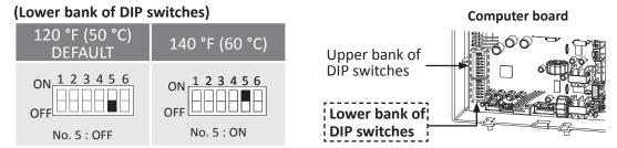
**NOTE:** The dark squares indicate the correct DIP switch positions.
