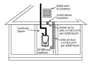
Figure 3 - Vertical duct openings
