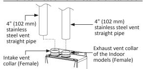
Connect 4" (102 mm) stainless steel vent straight pipes directly on the exhaust/intake vent collar of the water heater.
