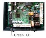
Error code on the computer board Indicated by 1/2-second flashes on the Green LED.
