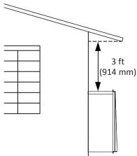
Ensure that you meet the minimum clearances shown below for a direct vent termination:
