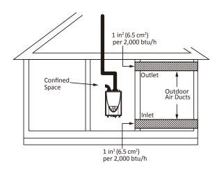
Figure 4 - Horizontal duct openings
