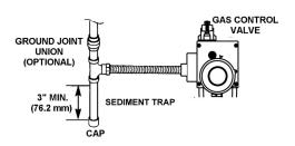
FIGURE 27. GAS PIPING WITH FLEXIBLE CONNECTOR
