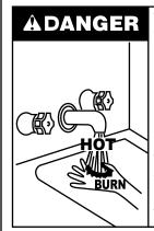
Water temperature over 125°F (52°C) can cause servere burns instantly resulting in severe injury or death.
