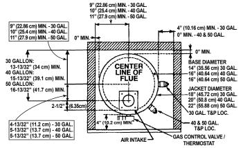
DIRECTION IN WHICH WATER HEATER CAN BE PLACED WHEN INCREASED SIDE CLEARANCE IS AVAILABLE
