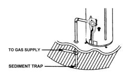
FIGURE 29. ALTERNATIVE SEDIMENT TRAP LOCATION
