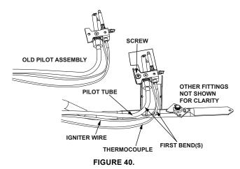
Route the new pilot tube and wires through the opening in the
