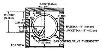
DIRECTION IN WHICH WATER HEATER MUST BE PLACED WHEN MINIMUM CLEARANCES ARE USED (30 GALLON ONLY)
