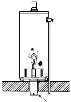
IF ATTACHING INLET PIPING, REMOVE AND DISCARD SCREWS AND WIND BAFFLE
