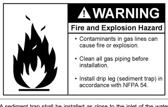
A sediment trap shall be installed as close to the inlet of the water heater as practical at the time of water heater installation. The sediment trap shall be either a tee fitting with a capped nipple in the bottom outlet or other device recognized as an effective sediment trap. If a tee fitting is used, it shall be installed in conformance with one of the methods of installation shown in Figures 28, 29, and 30.
