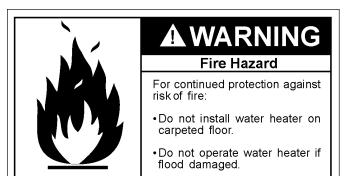
This water heater must not be installed directly on carpeting. Carpeting must be protected by metal or wood panel beneath the appliance extending beyond the full width and depth of the appliance
